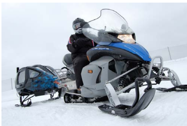
Figure 1. In-Service emissions analyzer being pulled by test snowmobile
