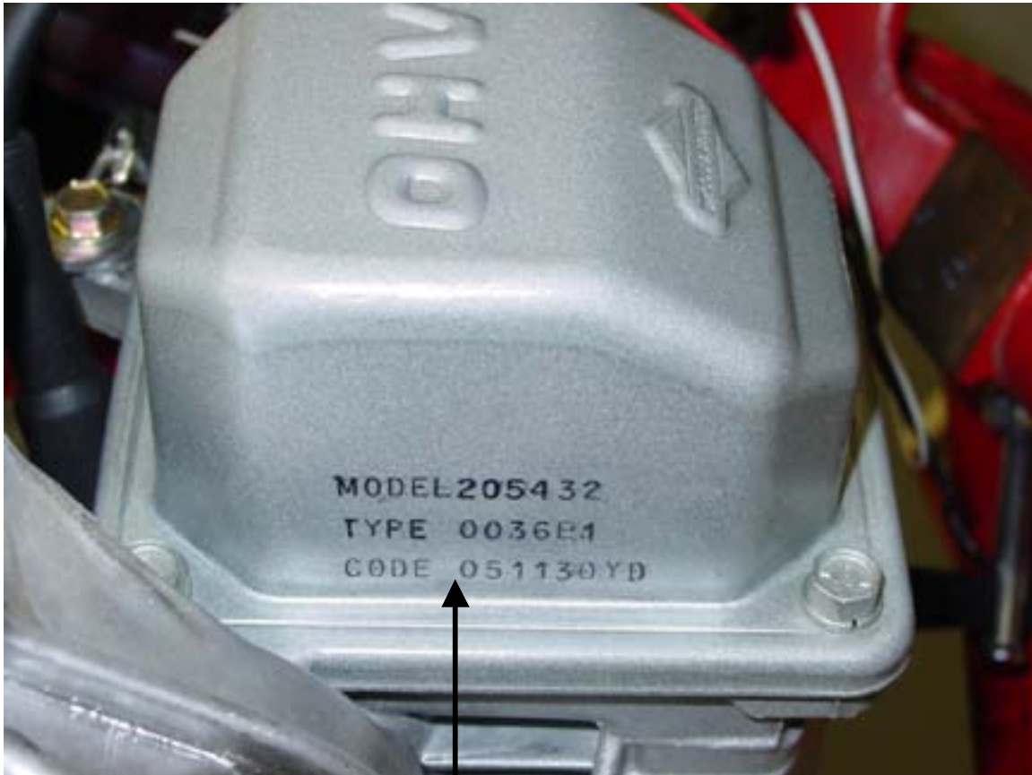
Engine model and type numbers are stamped into the engine valve cover.
