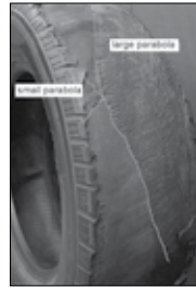
Fig. 1.4 Large and small parabolic separations joined across the casing.
